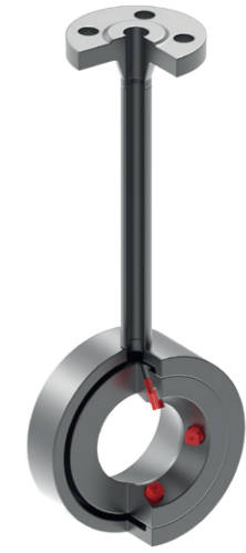
Steam cooler design utilising auxiliary steam to atomise injected water
